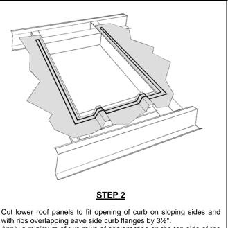
with ribs overlapping eave side curb flanges by 31/2". Apply a minimum of two rows of sealant tape on the top side of the roof panels.
