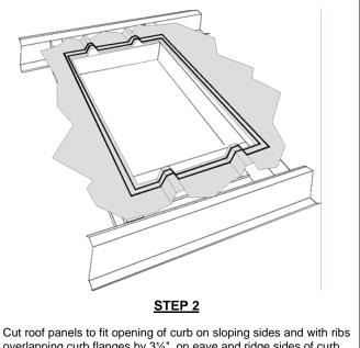
Cut roof panels to fit opening of curb on sloping sides and with ribs overlapping curb flanges by  $3\frac{1}{2}$ " on eave and ridge sides of curb. Apply a minimum of two rows of sealant tape on the top side of the roof panels.
