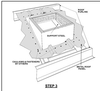
Fasten roof panel through curb flanges to support steel using suitable fasteners compatible with roof system. A minimum of four fasteners per side spaced on 6" centers or less as roof system permits. Fasteners should withstand a minimum pullout force of 160 pounds each.
