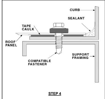
Inspect installation and fasteners. Apply sealant to seams around all sides of curb to assure a watertight seal.
