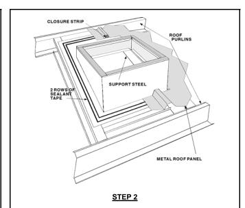
Cut roof panels to fit snugly around curb walls and to within 1" of the water diverter.
