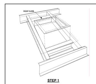
After building framing is complete, locate roof opening and install support framing for roof curb and equipment loads in accordance with building engineer's specifications. See "TYPICAL FRAMED OPENING DETAILS" sheet for recommended X and Y dimensions.
